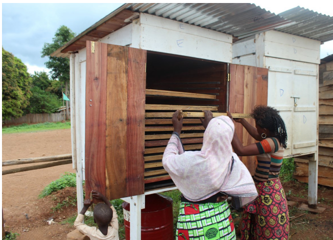
Efficient fish smoking kilns use up to 80-90% less fuelwood compared to the traditional open-fire method. Photo: Matis (Tanzania)
